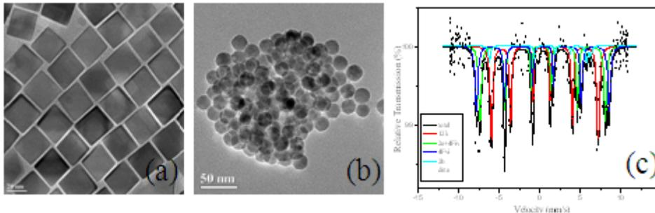
Fig.1. (a) TEM micrograph of 21 nm hematite nanocubes and (b) TEM micrograph of S-BaFe nanoparticles, and (c) Mössbauer spectrum of 20 - 25 nm sized S-BaFe particles.
