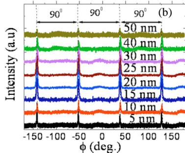
Fig.1 (a) XRD and (b)  $\phi$  scan for FePt/FeRh (50nm) bilayers with various  $t_{\text{FePt}}$  thickness.
