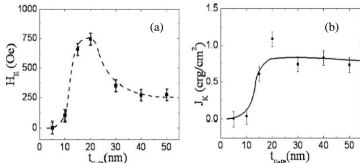
Fig.3 Exchange bias field  $H_E$  and Unidirectional anisotropy constant  $J_K$  for FePt/FeRh(50nm) bilayer.
