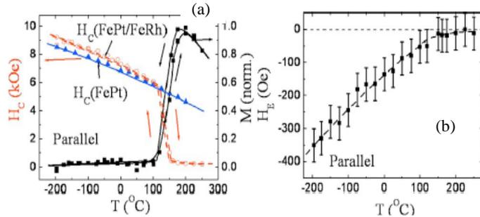
Fig.2(a)  $H_c$  and  $M$  vs  $T$ . (b)  $H_E$  vs  $T$  for FePt(50)/FeRh(50)
