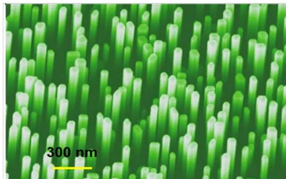
Figure 1. ZnO nanowire arrays growth on GaN substrate with diameters are around 50 nm and 300 nm to 2 micrometer in length.
